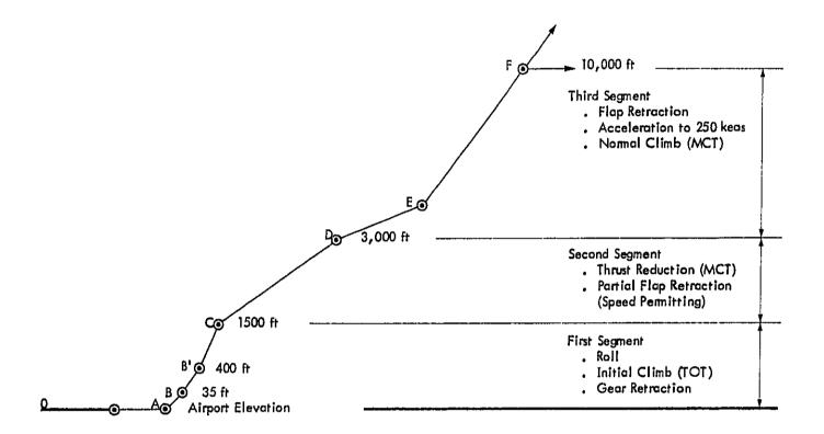
Figure 3.5-1. AC91-39 Flight Profile Illustration
